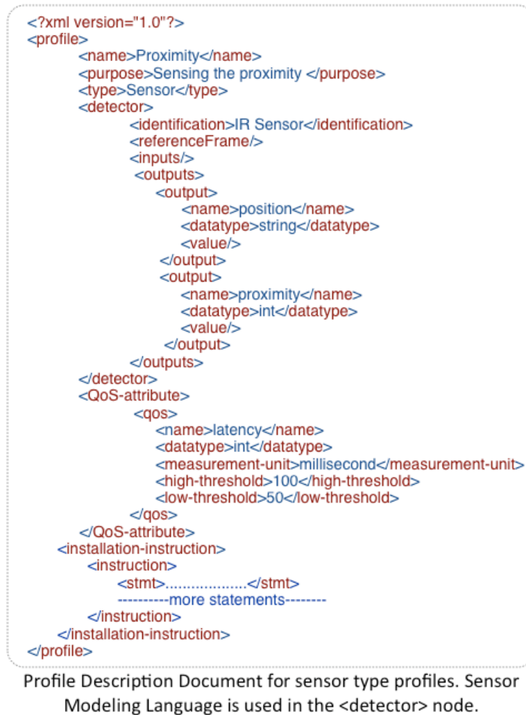
FIGURE 4.7: Profile Description Document for a sample Proximity Profile , Customized SensorML is used in the detector node.
