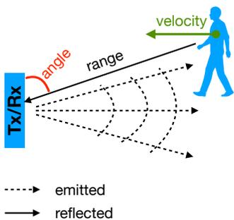
**Figure 1:** Radar sensing system.
